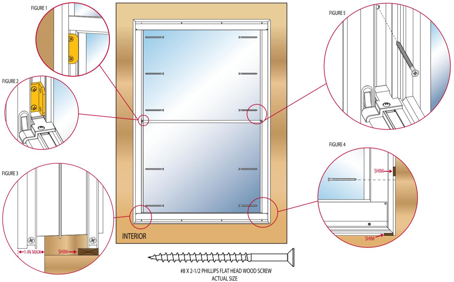
With the panel standing upright, remove and discard the three metal shipping clips. Two are located under the bottom of the top sash on the outside of the panel. One is on the inside on the top of the bottom sash, near the sash lock. (Figures 1 & 2)
